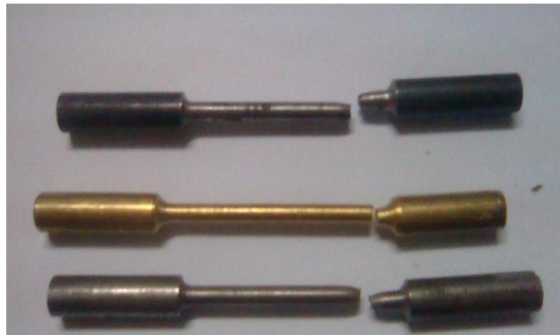
Figure 6. Photograph of Specimens Prepared According to the ASTM E8 Standard.
